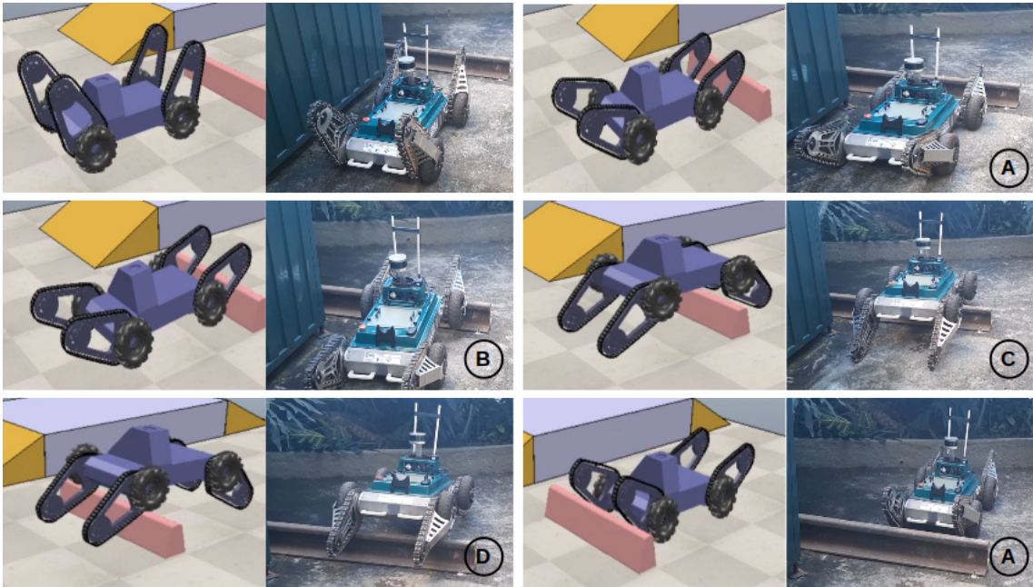
Figure 5.28: Robot sequence to climb a rail, on the simulation environment and reality.
