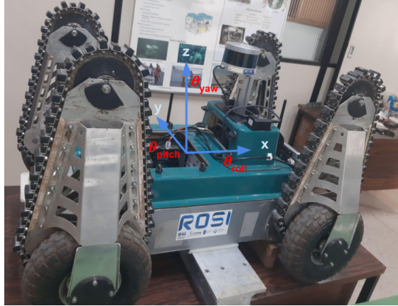
Figure 5.2: Rosi mobile robot used to test the LIO-SAM framework.
