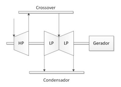
Figura IV.22 – Turbina tandem-compound – TKCSA.
