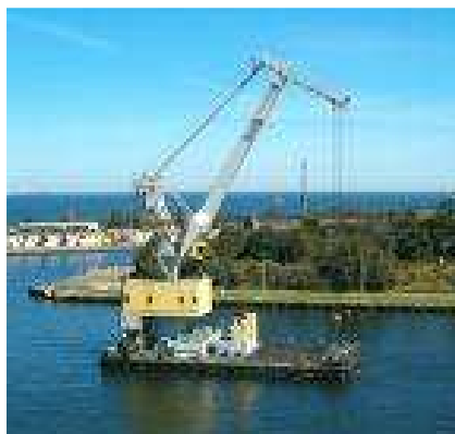
Figura 2-5 Floating Crane (Balsa Grua)
